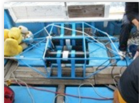
Deep water (6000m) Extended Range 300KHz ADCPs ready for deployment
